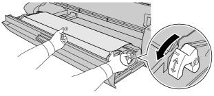
6 Rotate the roll holder in the direction of the arrow until the edge of the roll media reaches the edge of the paper guide.
